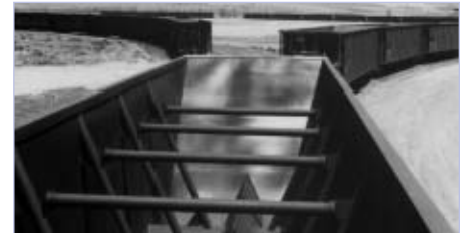
Basin Electric railcars with TIVAR® 88-2 liners installed.
